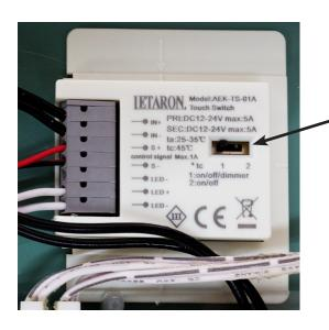
Your illuminated mirror offers the option of switching between the dimmable version and the non-dimmable version. To do this, screw on the switch box (photo above) on the back. There is a switch in the module (see left). In position 1, the dimmer is switched on. In position 2, the touch switch only works in ON/OFF mode.
